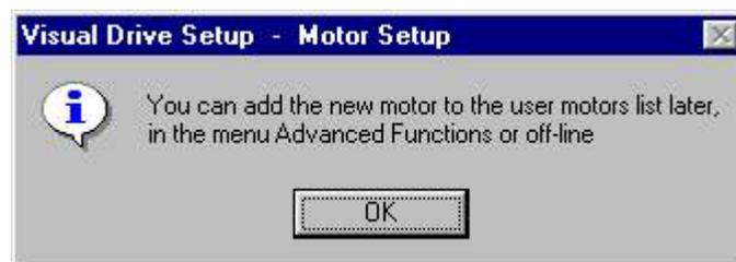
The identification of this new motor can be entered at any time by selecting **Add new motor in user list**, in order to include it in the user motor list.
