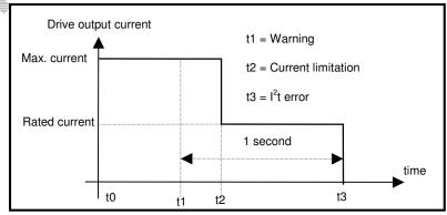
The maximum current duration before release of the warning is depending on the value of the parameters Rated current and Max. current. This value is calculated as follows:
