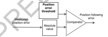
The measured position error value is continuously compared with the the **Position error threshold** parameter value. When the measured position error is exceeding the **Position error threshold**, the position following error is released. This configuration is used for applications requiring the smallest possible following error.
