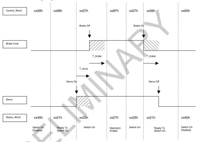
T\_brake Motor Brake Reaction Time
