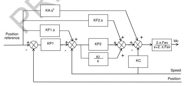
**Speed error low-pass filter (Fev)**: defines the cut-off frequency at -3dB of the first order filter which acts on the current command (ldc). This value is calculated by the amplifier during the auto-tuning procedure and depends on the selected bandwidth and the selected filter type.
