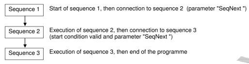
If the execution is starting at sequence 1 and logic input 8 is desactivated, the programme will be the following:
