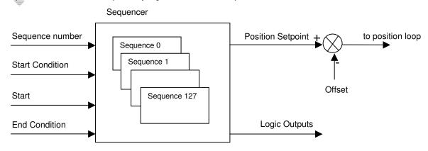
**Sequence Number**: allows to select the sequence to be executed. The "Sequence Number" can be connected to physical logic inputs or set via field bus to select the sequence.
