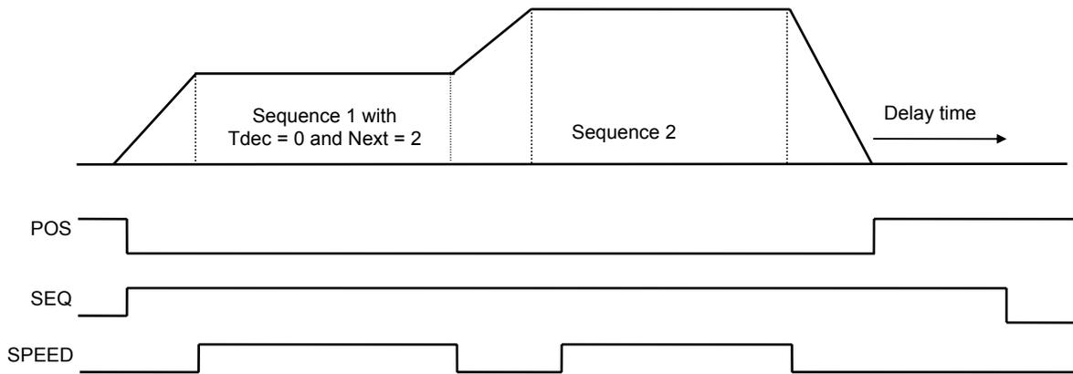
**OUT1 to OUT4** Programmable logic outputs. These outputs are only operating during a programmed sequence.
