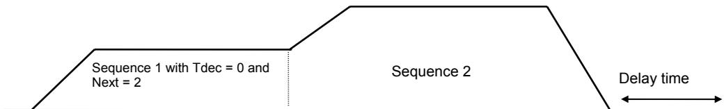
**Note:** For a small displacement, when the programmed motion speed value cannot be reached, the motion speed profile is modified according to the **Profile limit** parameter selection:
