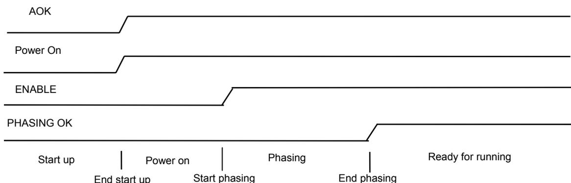
In the Profibus mode, the phasing procedure must be started by the master controller (PNU 896). In the Software control mode via the serial link, the phasing procedure must be started by the Motor phasing command in the **VDS**Setup window.
