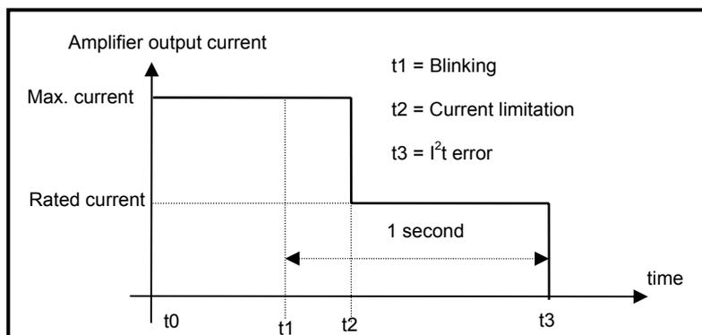
The maximum current duration before release of the blinking display is depending on the value of the parameters **Rated current** and **Max. current**. This value is calculated as follows:
