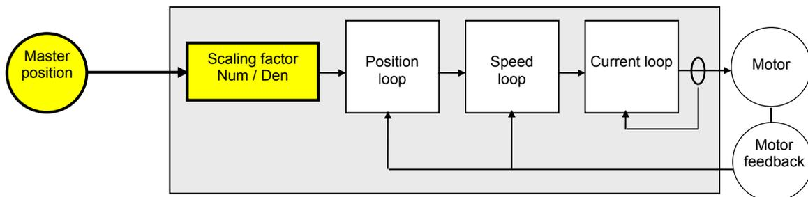
Electronic gearing applications require the use of the second amplifier position sensor for measuring the displacements of the master axis.
