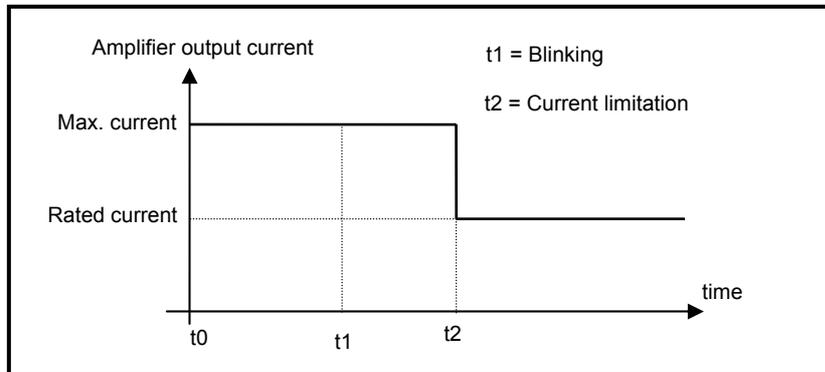
The maximum current duration before release of the blinking display ( $t_1 - t_0$ ) and before limitation at the rated current ( $t_2 - t_0$ ) is calculated the same way as in the "Fusing" mode.
