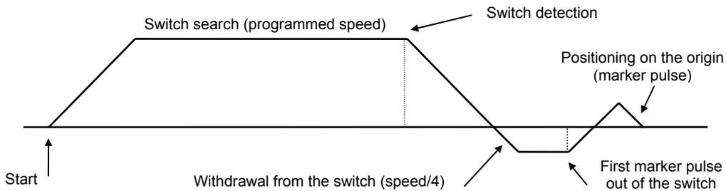
If Switch=1 and Zero=1 or Home=1, the speed can be reversed by the switch detection or by a limit switch.
