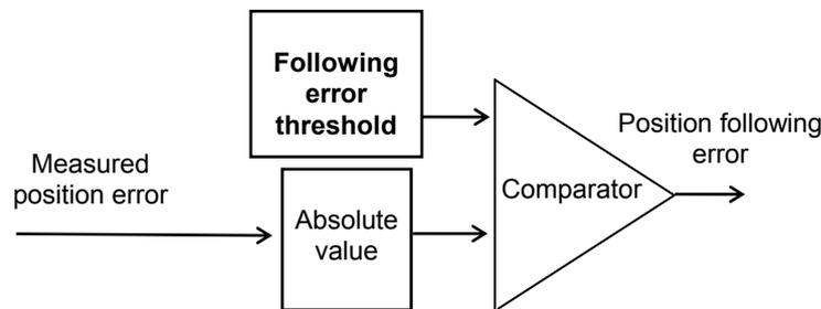
The measured position error value is continuously compared with the the **following error threshold** parameter value. When the measured position error is exceeding the **following error threshold**, the position following error is released. This configuration is used for applications requiring the smallest possible following error.
