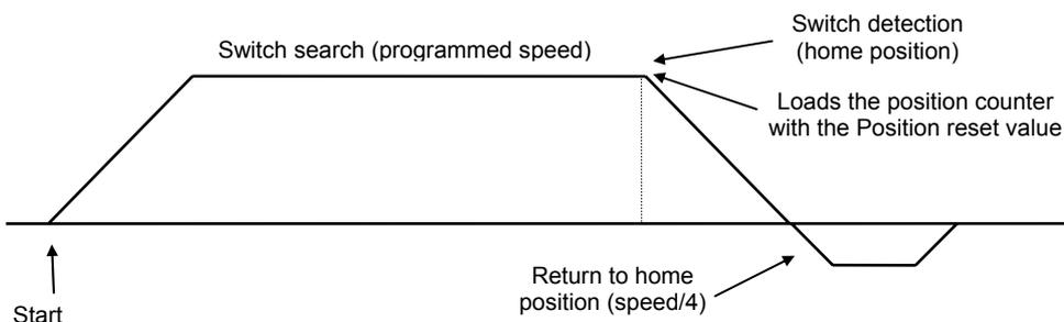
When sequence 0 contains a homing procedure at power on, no other sequence can be executed before sequence 0.
