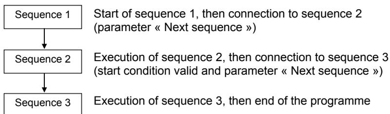
If the execution is starting at sequence 1 and logic input 8 is deactivated, the programme will be the following:
