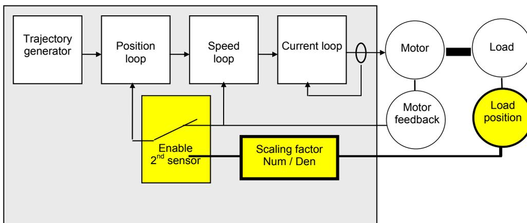
Resolver sensor feedback for the motor, and TTL incremental encoder for the second sensor is the default configuration.
