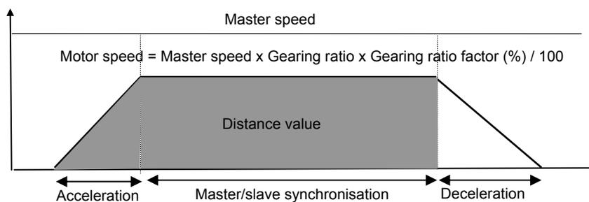
The acceleration and deceleration times parameters define the time with regard to the **Maximum Speed** parameter value as in a positioning sequence or a homing sequence.
