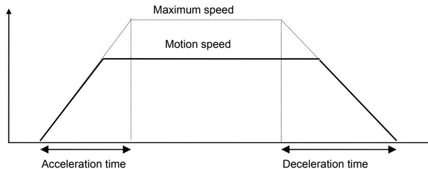
Remark : The JOG deceleration time parameter value is also used when the STOP input is activated.
