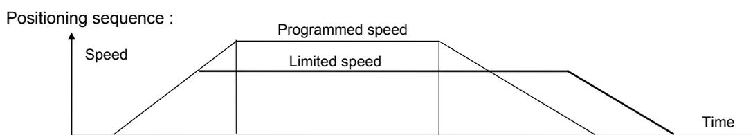
**Enable speed modulation:** when this command is selected, the programmed speed can be modified on-the-fly (during the sequence execution) for a positioning sequence (ABSOLUTE or RELATIVE). For the other sequences, the programmed speed is limited during the whole sequence execution according to the limitation value at the sequence start.
