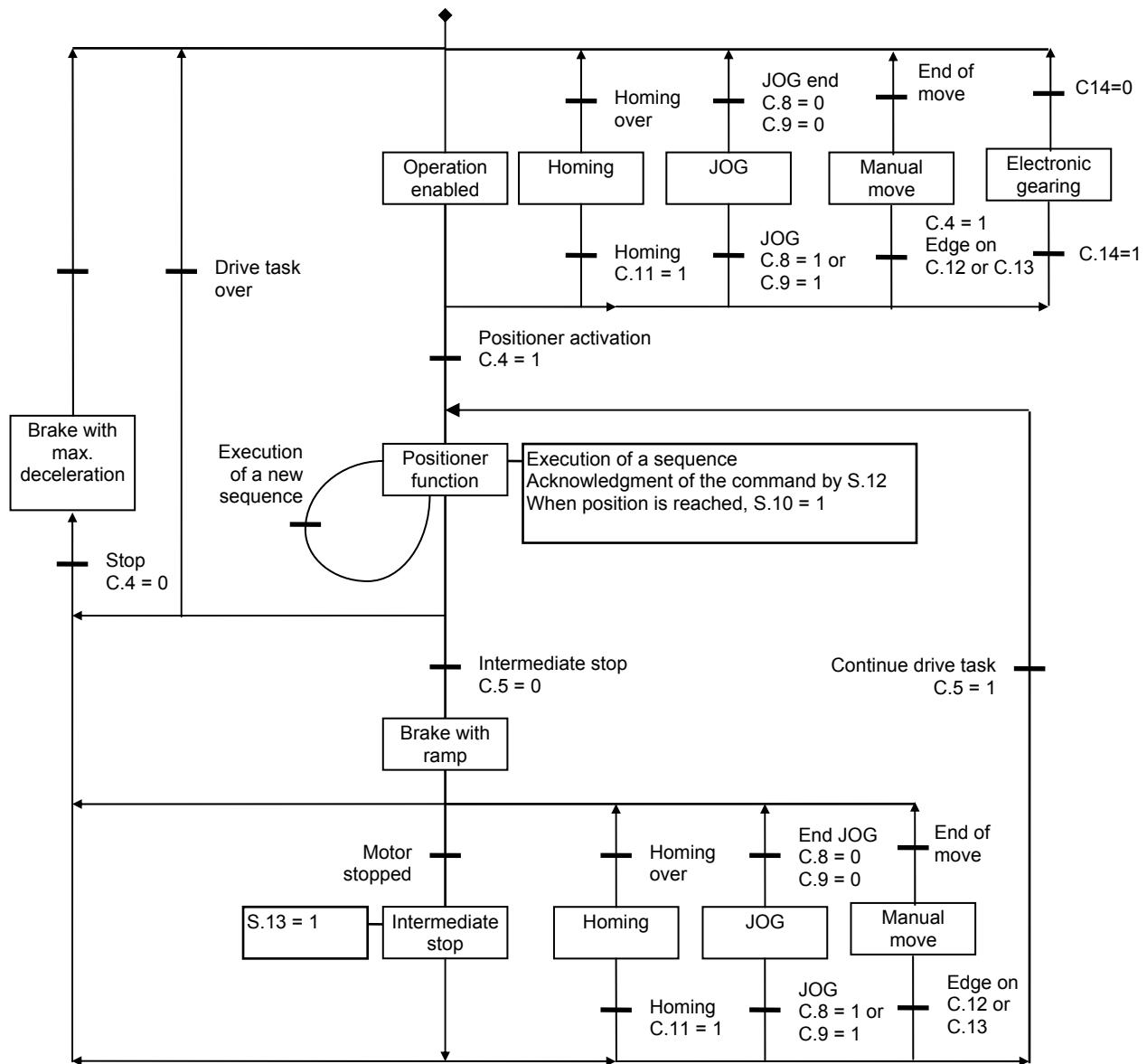
When the positioner is in "Operation enabled" status, the following actions are possible:
