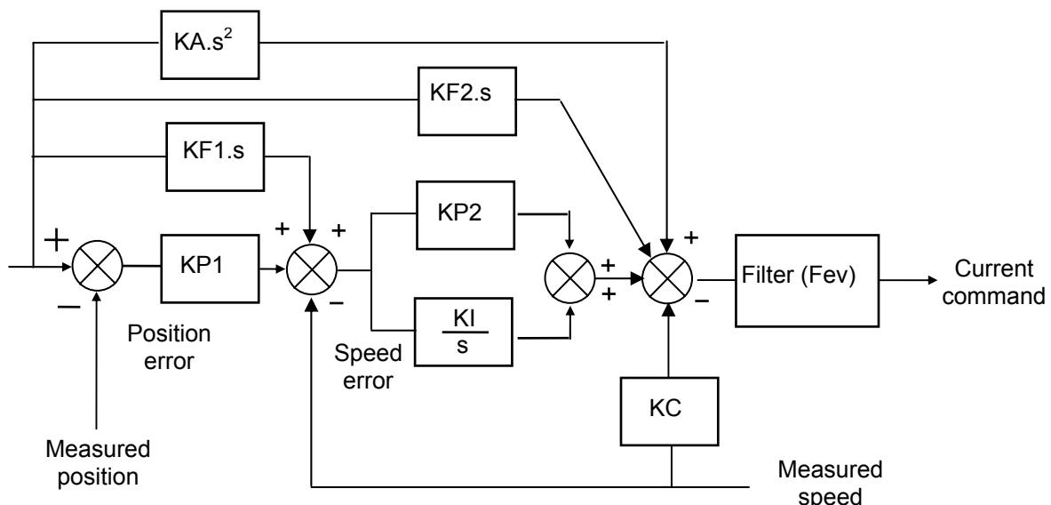
All gain parameters (KF1, KF2, KP1, KP2, KI, KA, KC and Fev) are automatically calculated during the auto-tuning procedure.
