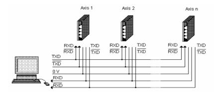
All amplifiers are parallel connected to the computer.
