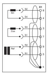
For the use of **resolvers** with **transformation ratios** out of the range 0.3 to 0.5, the adjustment must be factory set by INFRANOR.
