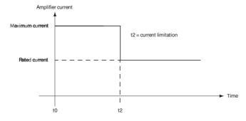
The maximum current duration before limitation at the rated current (t2 - t0) is calculated the same way as for the **Fusing** mode.
