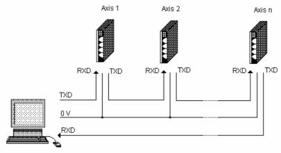
The connection of the various units (host PC and amplifiers) is made as a ring: the transmission signal (TxD) of each unit is connected to the reception signal (RxD) of the next unit. Each CD1-a amplifier has got 4 microswitches allowing an address assignment. The CD1-a amplifiers inside the ring must have different addresses. An address in multi-axis configuration must have a value between 1 and 15. The 0 address corresponds to the single-axis communication configuration (no addressing).
