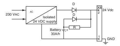
The CD1-a amplifier consumption is 320 mA with 24VDC. So, a 24 V / 30 A/h battery can keep the amplifier on during i.e. a long 3 days week-end or during a mains cut-off without loosing the machine initialization. This backup method is very interesting for saving the machine initialization as well as the axis position even when moving with the mains switched off. An ASCII command allows to send the axis position to the digital host system.
