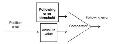
The position loop error value is continuously compared with the value of the **Following error threshold** parameter. When its value is exceeding the one of the **Following error threshold** parameter, the following error is released.
