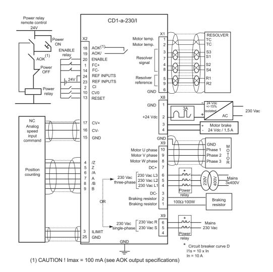
The protection, on source side, of both 24 V and power supplies must be made by the user.
