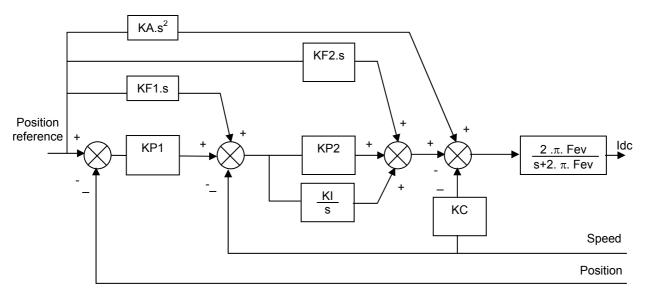
Speed error low-pass filter (Fev): defines the cut-off frequency at -3dB of the first order filter which acts on the current command (Idc). This value is calculated by the amplifier during the auto tuning procedure and depends on the selected bandwidth and the selected filter type.
