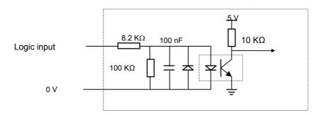
The input voltage corresponding to level 1 is between 18 V and 30V.
