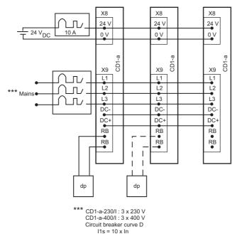
For a multiaxis application with n drives, the circuit breaker rating is given by
