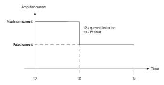
The maximum current duration before limitation at the rated current is depending on the value of the **Rated** current and **Maximum current** parameters.
